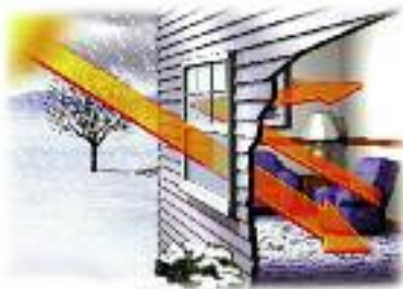
Low-E glass takes on a new duty in winter months. It lets warm solar rays into your home preventing indoor heat from escaping.
